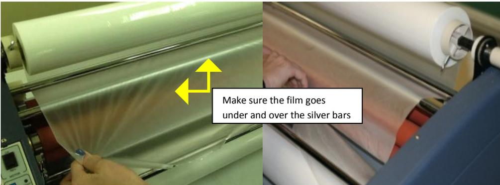
2) Pulling the film through the rollers you need to make sure the film is perfectly aligned at top and bottom. Note: overlap will cause the film to deposit adhesive on the rollers. To thread, you can see the "threading card" that was supplied with the machine.
