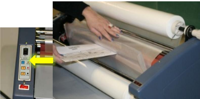
3) You can now power the machine ON by pressing the red power button. Once you insert the threading card in between the rollers and press the ON motor switch the film will thread through the machine.
