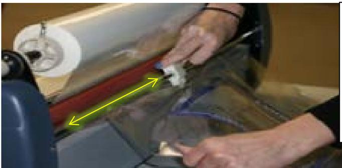
6) You are now ready to laminate! Simply place your desired documents on the feed tray, press the motor ON button, and allow the machine to pull document through. The finished product will come out the back of machine and you can use the attached film splitter to cut at your desired position.
