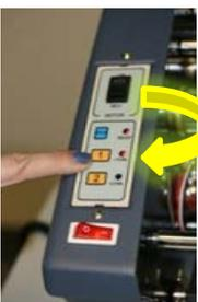
4) Now your machine is ready to begin heating. You do this by pressing either the "1" button for 1.5mil or the "2" button for 3mil, depending on the thickness of your film. Optimal heating time is 10-12 minutes to ensure a perfect lamination. You will know this is ready when the blinking light becomes solid.
