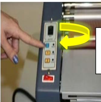
7) Upon completion of lamination, press the blue "COOL" button to turn off the heat. Once the rollers have cooled off you can now turn the power switch OFF.
