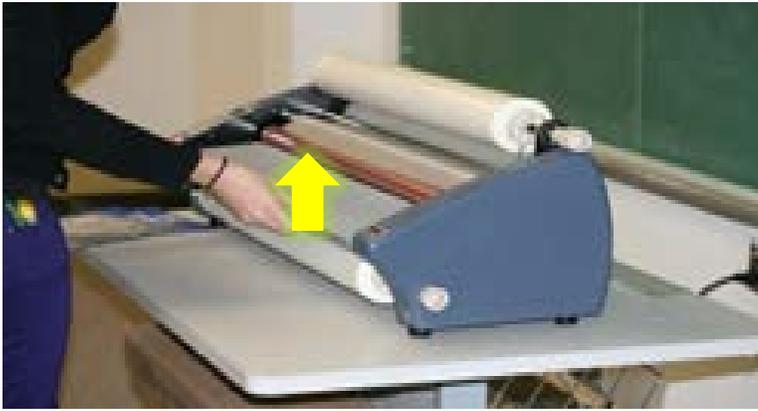
5) Place the feed tray and guide plates on holders above the bottom roll
